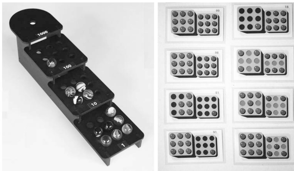
Figure 6-2. The Marbles Calculator and 100-cards. In the card version the marbles were color coded: red for ones, green for tens.
