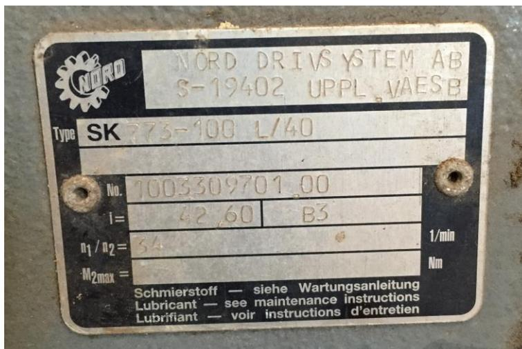
Figure 4.14 Rating plate on the gearbox.
