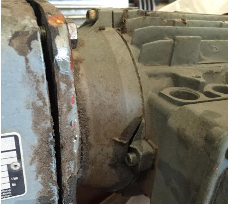
**Figure 4.15 Damaged flange connection.**
