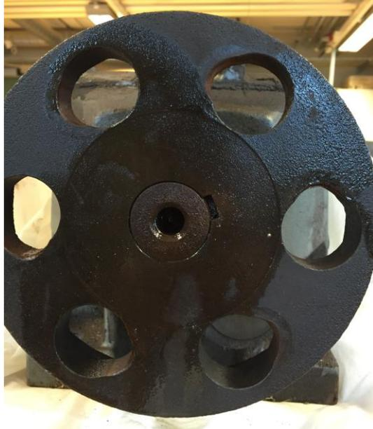
**Figure 4.17 Pulley on the output shaft of the gearmotor.**
