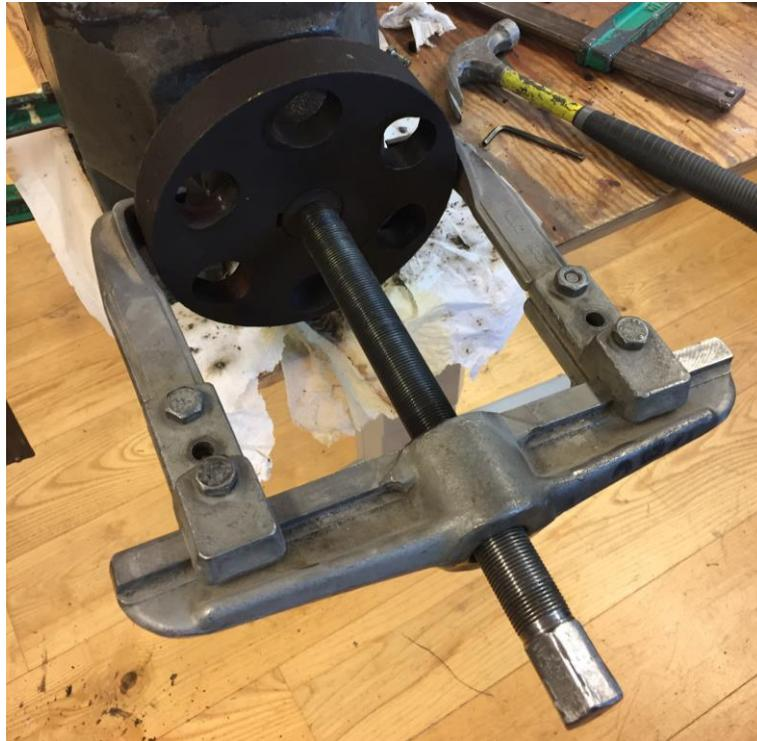
**Figure 4.19 Attempting to remove pulley with gear puller.**
