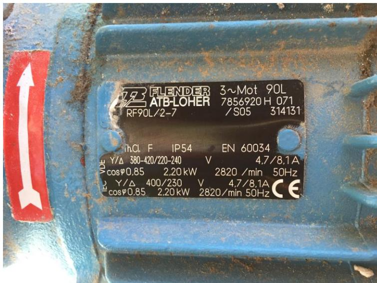
**Figure 4.5 Rating plate of the motor.**
