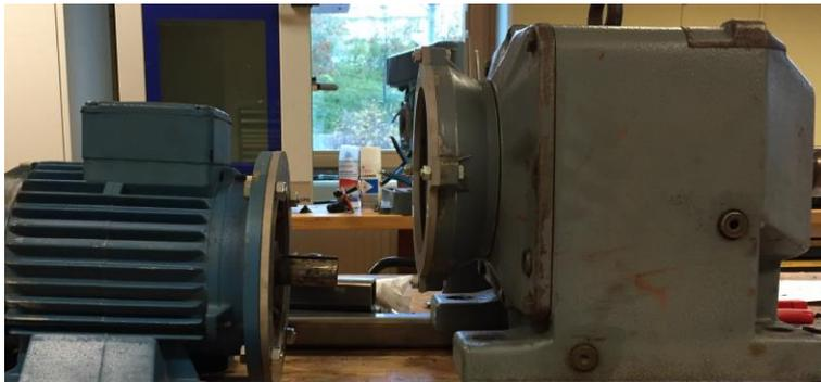
**Figure 4.23** PSU configuration after removing the rotor with the remaining shaft connected to the gearbox.
