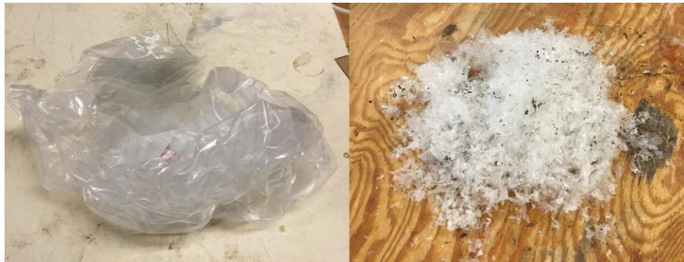
**Figure 5.3 LDPE-film before and after being shredded without a sieve.**
