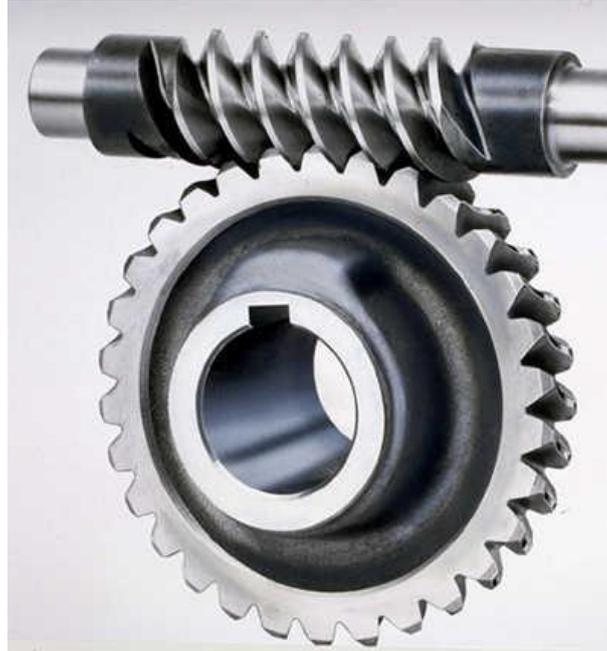
**Figure 4.8 The basic setup of a worm gear.**
