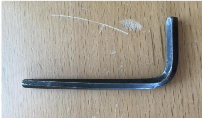
**Figure 4.18 Allen key twisted from trying to remove the set screw.**
