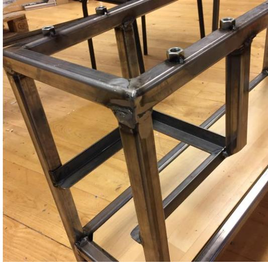
**Figure 6.17 Slide rail for a smaller collector.**
