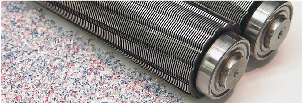
**Figure 3.7 Paper shredder with hook knives.**
