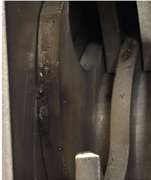
**Figure 6.10 Splashed beads of metal from welding the sieve to its supports.**
