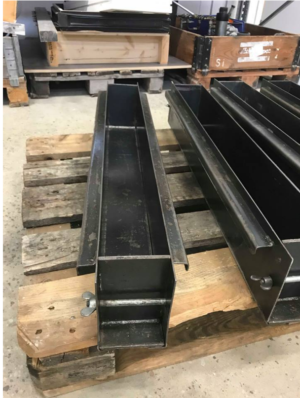
Figure 25: Mini steel form for beam size D
