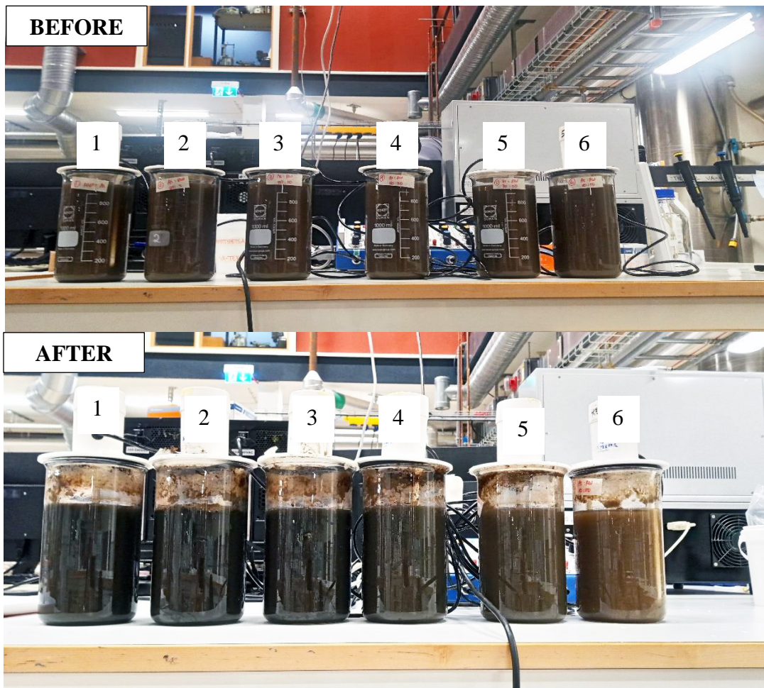
Figure 4.9. Before and after hydrolysis Experiment 2, the diffuser attachment successfully eliminates the spilling problem.
