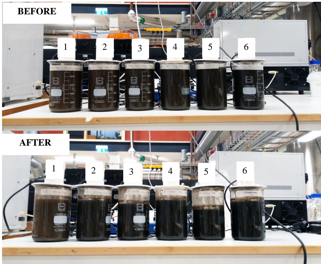
Figure 4.1. The before and after hydrolysis and the spilling problem that happened in the jars.
