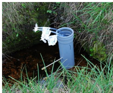
Figure 3 Pore water sampler (P1) was used to collect stream water sample. The photo was taken in the summer, 2011.
