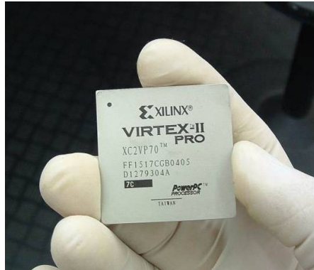
Figure 2.1 An FPGA circuit.
