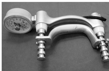
Figure 10. The Jamar dynamometer. The width of the grip is adjusted in five steps. Step 2 is the commonly used size.
