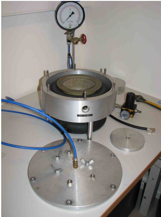
Figure 30 The Cembureau test equipment for measurement of gas permeability.
