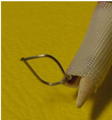
Figure 6 Welded thermocouple wire, diameter 0.5 mm.
