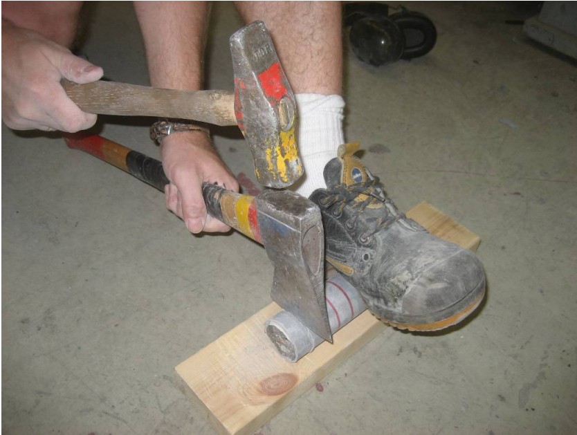
Figure 13 The author is slicing of the specimens where the notch is.
