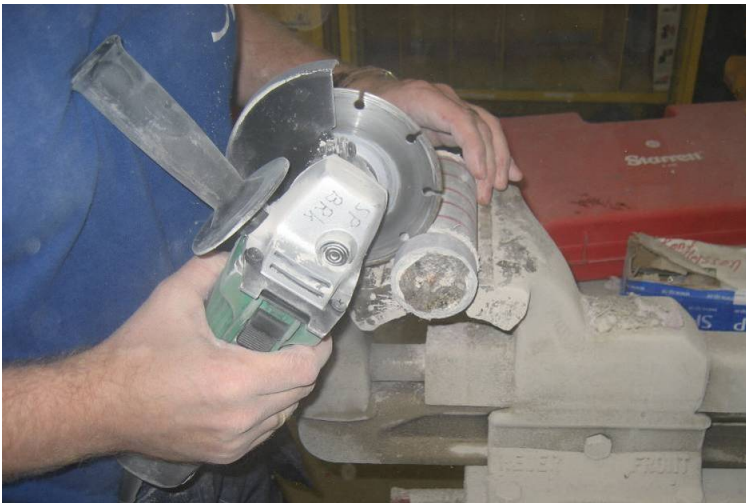
Figure 12 The author is notching of the specimens.
