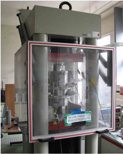
Figure 34 The equipment for measurements of mechanical properties at high temperature at CSTB in France.
