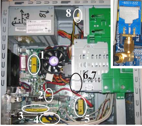
Fig. 1. An inside view of the HP computer. The eight circled Tx/Rx blocks (of various sizes) can be seen scattered over the computer. Block 6 is located in the horizontal plane, on the motherboard, whereas block 7 is located in the vertical plane, on the hard drive (around 7 cm above the motherboard). Also, inset in the top right corner is a (magnified) picture of the SMA connector) picture of the SkyCross antenna.
