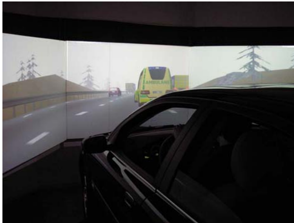
Fig. 1. Views of the simulator gaming environment: the driving simulator uses seven screens to project a nearly 360 degree-field, allowing the use of rear-view mirrors and side-views of surrounding traffic (from Backlund et al, 2007).
