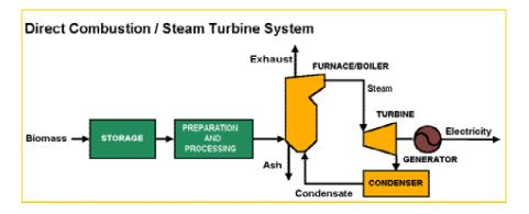
Figure 4: Direct combustion/ Steam turbine system. Source: Distributed Energy Resources (DER)
