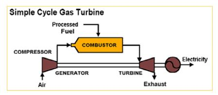
Figure 5: Simple cycle gas turbine. Source: Distributed Energy Resources (DER)
