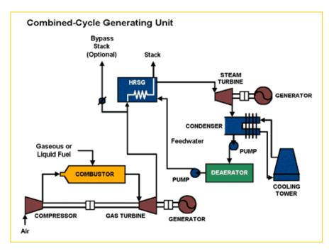
Figure 6: Combined cycle generating unit. Source: Distributed Energy Resources (DER)
