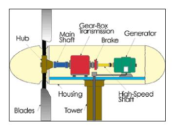
Figure 7: Components of a wind turbine. Source: Iowa Energy Centre (IEC)
