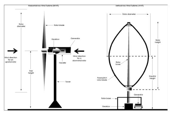
Figure 8: Two basic wind turbine configurations. Source: Cavallo, Hock and Smith (1993)
