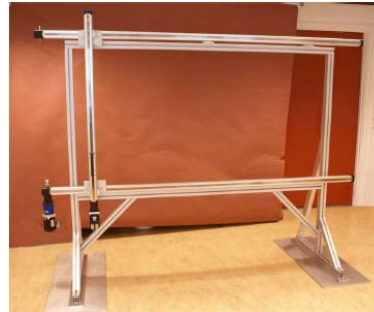
Fig.3. The experimental setup xy-table, with x and y travelling ranges of 2 and 1 meter, respectively.
