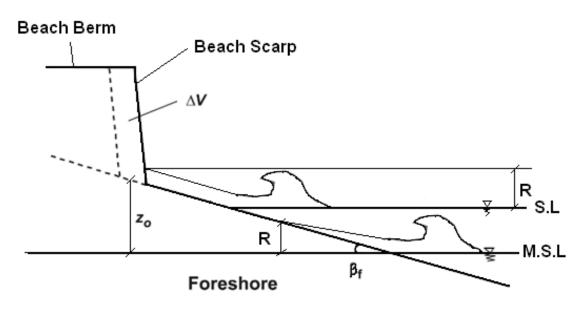
Figure 4.21 Schematic description of berm erosion due to wave impact in the presence of a scarp. (H. Hanson tvrl.lth.se)
