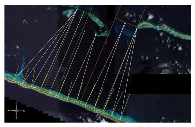
Figure 4.15 Shoreline sections of 1000 m with normal and diffraction angle. (IKONOS 2001)
