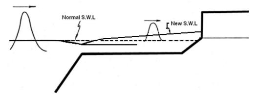
Figure 4.23 Example of wave set-down and wave set-up. (U.S. Army Corps of Engineers, 2002)
