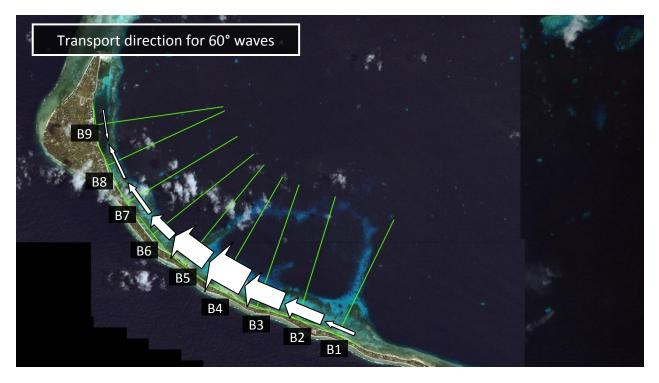
Figure 6.2 Sediment transport direction for incoming waves at 60°. (IKONOS 2001)
