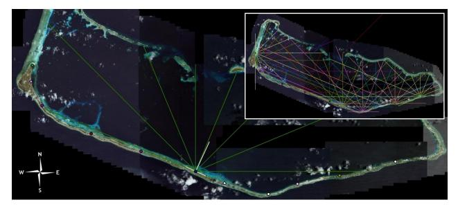
Figure 4.17 Example of fetch lengths for a location in the lagoon and an insert showing all fetch lengths. (IKONOS 2001)
