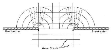
Figure 4.10 Example of wave diffraction in a harbor entrance. (Hanson, 2010)
