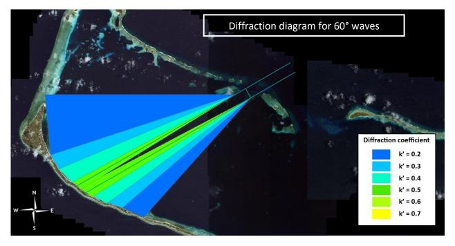
Figure 4.14 Diffraction diagram for correction coefficient k' for the small opening for 60° waves. (IKONOS 2001)
