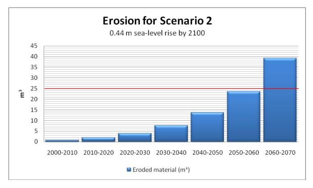
Figure 6.6 Erosion for Scenario 2 at Profile 8.
