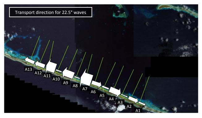
Figure 6.1 Sediment transport direction for incoming waves at 22.5°. (IKONOS 2001)
