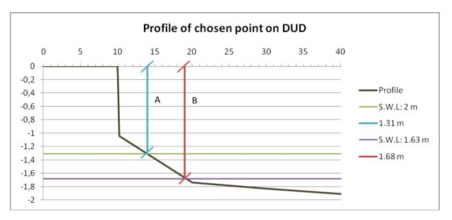
Figure 4.25 Profile of the chosen point on DUD for overtopping evaluation.
