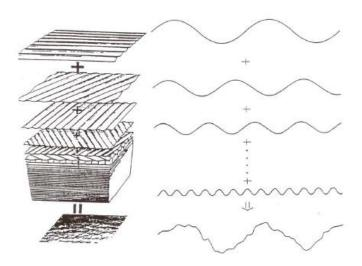
Figure 4.7 Example of a combined wave systems. (U.S. Army Corps of Engineers, 2002)
