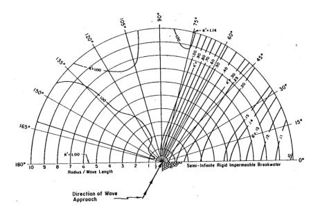
Figure 4.11 Wave diffraction pattern developed by US Army Corps. (U.S. Army Corps of Engineers, 2002)
