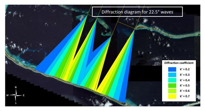
Figure 4.13 Diffraction diagram for correction coefficient k' for the openings for 22.5° waves. (IKONOS 2001)
