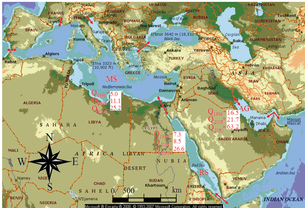
Fig. 1. Brine water Q_B results in 10^6 \text{ m}^3/\text{d} for the Arabian Gulf (AG), Mediterranean Sea (MS), and Red Sea (RS) in 1996, 2008, and 2050 (map from: Google Earth)
