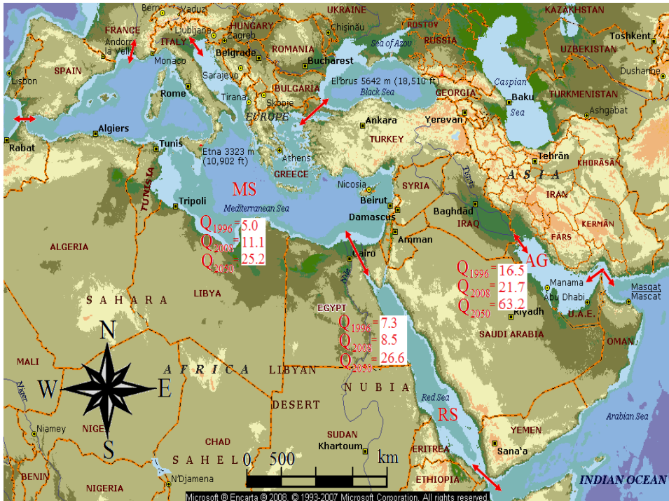
Figure 2.1 Brine water Q_B results in 10^6 \text{ m}^3/\text{d} for the Arabian Gulf (AG), Mediterranean Sea (MS) and Red Sea (RS) in 1996, 2008 and 2050 (map from: Google Earth)
