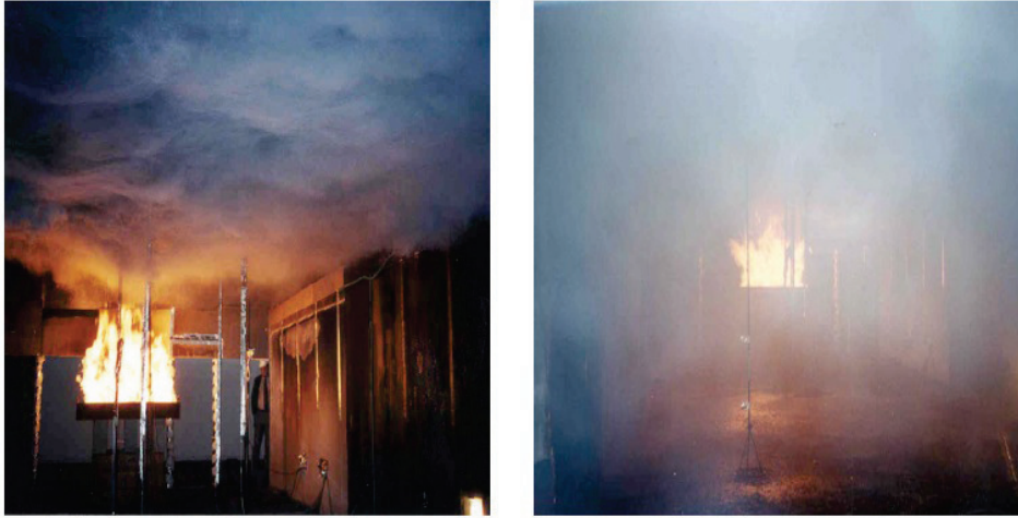
Figure 6.3 Smoke layer characteristics, prior and after sprinkler actuation (Kumar, 2006).
