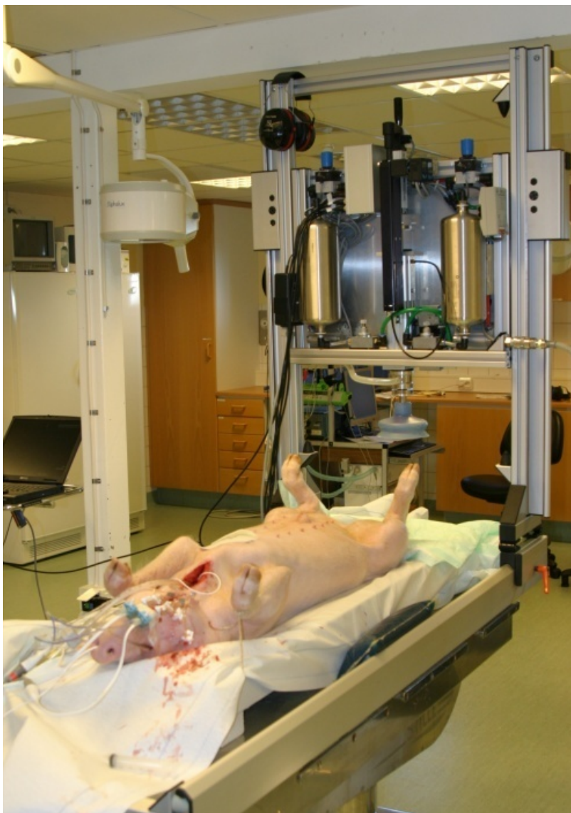
Fig 3. The Universal Igelösa research machine constructed to study all parameters of mechanical chest compression and active decompression on all sizes of animals.
