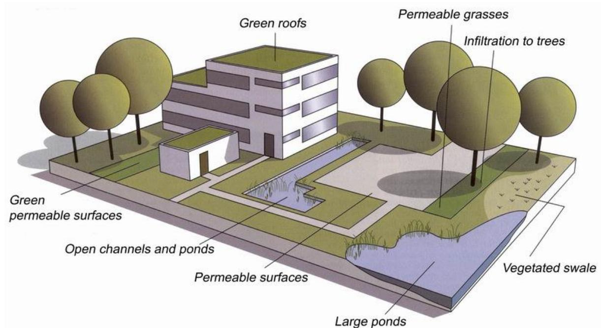
**Figure 5.** Urban stormwater management. Source: Veg Tech.
