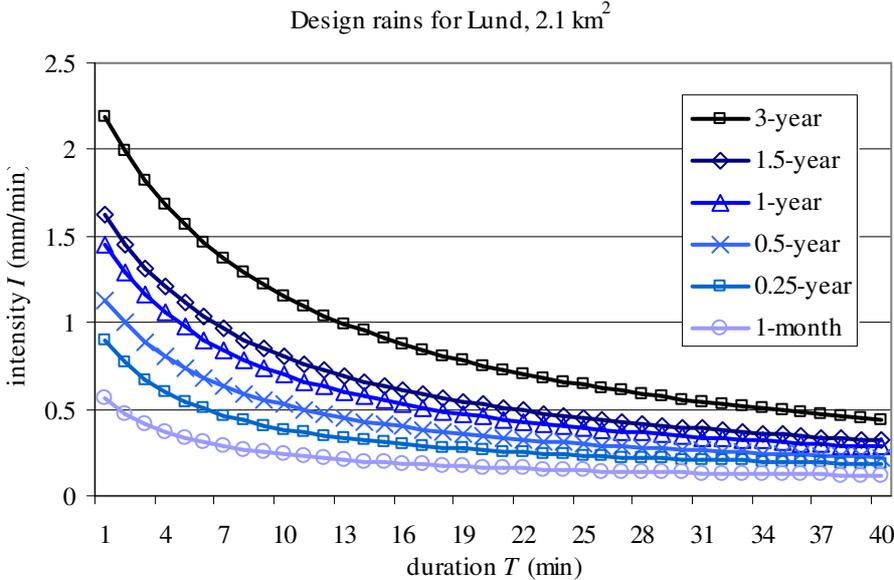
**Figure 8.** Design rains for Lund. Intensity as a function of duration, where curves show the mean intensity for a rain of a particular duration.
