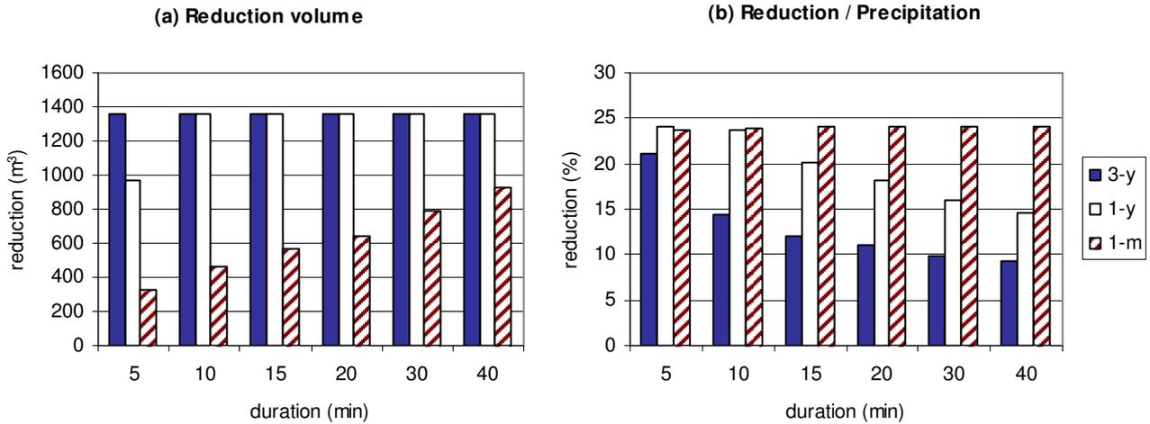
**Figure 11.** Volume reduction in thousand  $m^3$  (a) and share of total precipitation (b) for total area with the use of green roofs. Initial water levels are 50%. Design scenarios for 3-year, 1-year and 1-month rains are presented.
