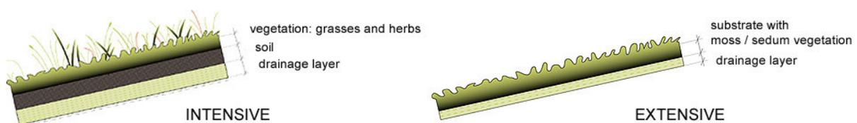
**Figure 4.** Typical buildup of a green roof. Intensive and extensive are similar, but intensive have other types of vegetation. They also require a roof that can hold more weight since they need more storage of water and thus have thicker layers. Source: Veg Tech.
