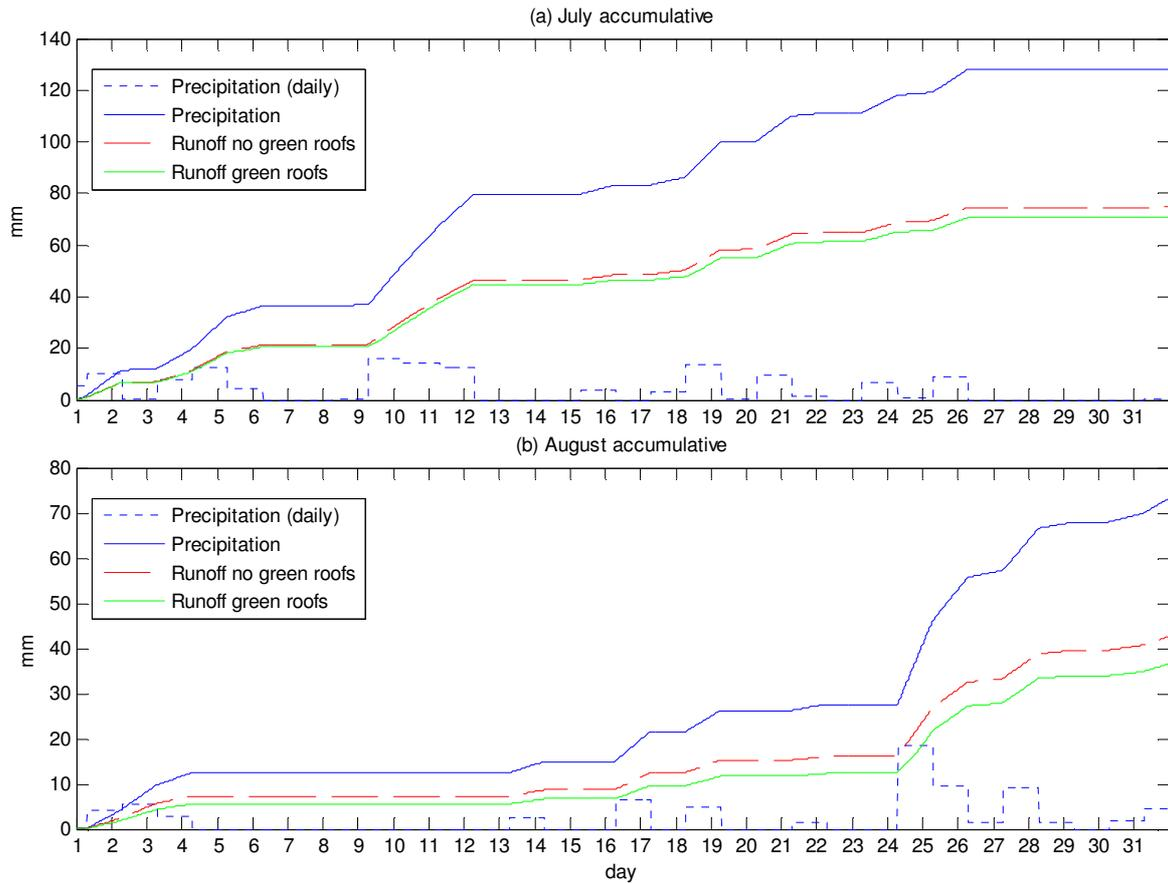
**Figure 17.** Accumulated precipitation and runoff with and without the use of green roofs for study area under July (a) and August (b). Note the different scaling on the y-axis.
