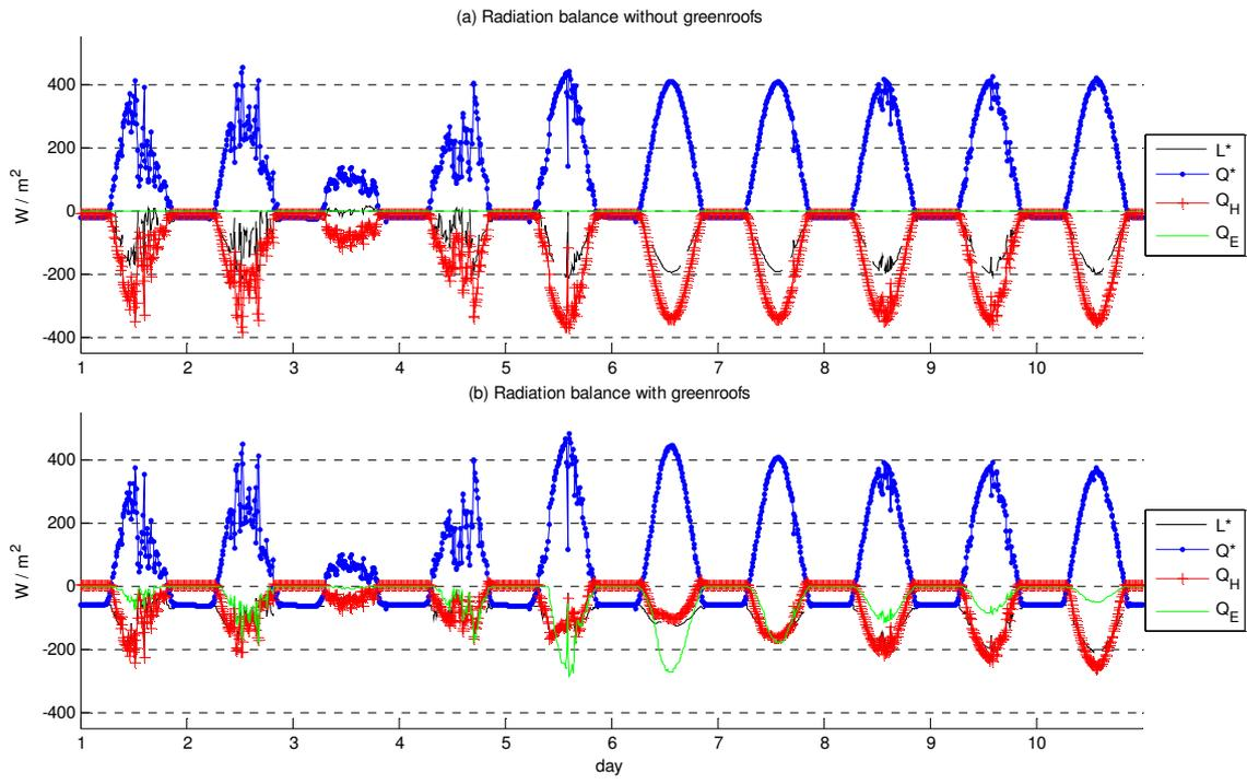
**Figure 12.** Excerpt of monthly simulation for 10 days in August without (a) and with (b) green roofs.
