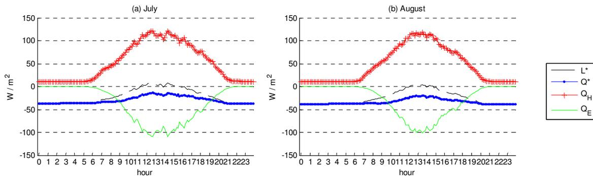
**Figure 16.** Green roof impact on radiation balance for July (a) and August (b). Values shown are changes brought from green roofs.
