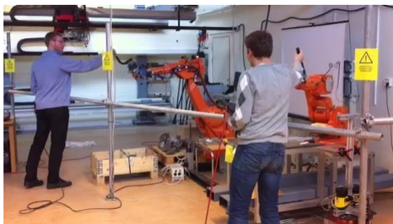
Figure 10.1 Lead-through of virtually connected robots.
