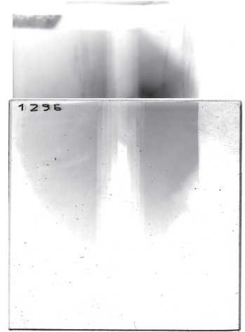
Figure 6.6. Comparison between a profile acquired with the scintillator and a CR-39 detector. The shadow of metallic filters with different thicknesses are visible, providing a rough energy measurement.
