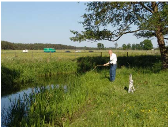
Fig. 1.5.1. The river site of Klingavalsån where several campaigns were carried out. In the background several vehicles can be seen, the white trailer is a 40 kVA diesel power plant powering the lidar. The mobile lidar itself is constructed in a green Volvo truck. In the foreground, Prof. Sune Svanberg is communicating with the operators in the lidar while producing a fluorescence return echo from a stick for signal optimization.
