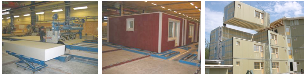
FIG 2: Modular house production
