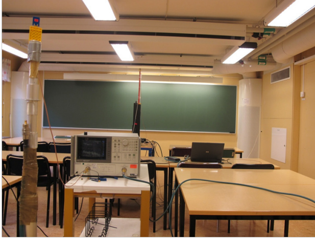
Figure 9.4: Overview of the measured scenario. Tx antenna in front and Rx antenna in the back.
