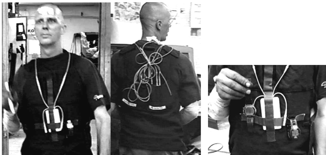
Figure 5. To the left - inclinometers to measure head, upper back and arm postures applied on a disassembly worker's forehead, neck and upper arm. Figure 6. To the right - goniometer placed on a disassembly worker's right hand.
