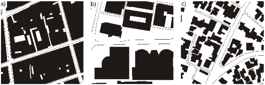
Fig. 2.12 Footprint area of buildings and road network in (a) the old commercial quarters (Pettah), (b) the central business district (Fort) and (c) a residential suburb (Nugegoda). Map size: 200 m × 200 m.
