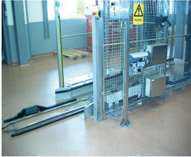
Figure 8. The RFID reader at the gate of the roll container washing machine.
