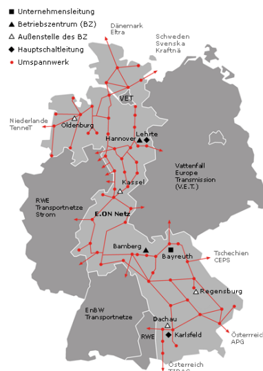
Figure 3.7 The control area of E.ON Netz GmbH.
