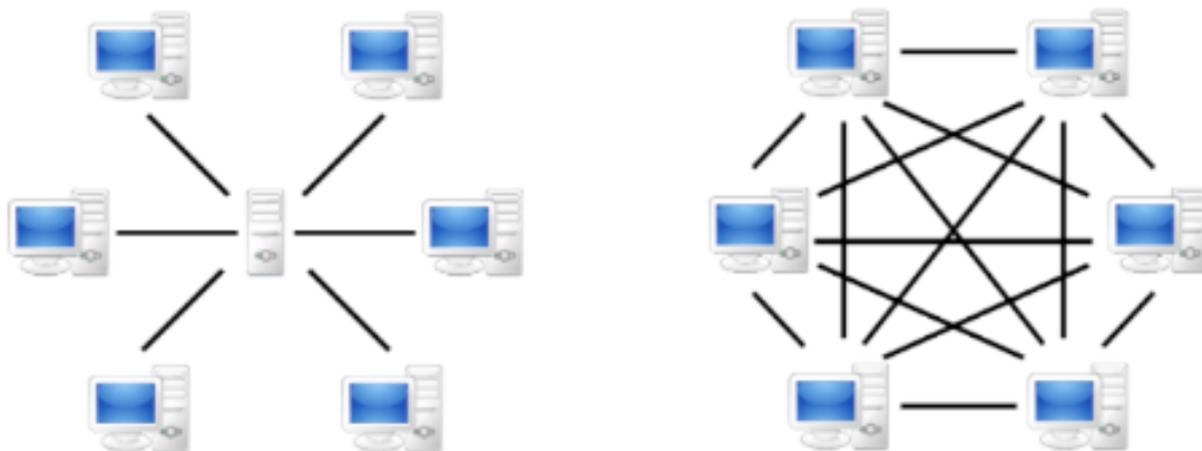
Figure 1. A one-to-many network: where a central server controls and distributes information, (left). A peer-to-peer network: where every node is both a client and a server, sharing information, (right). (Gigatribe, n.d.)
