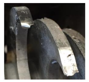
Figure 5.6 Chipping of the teeth after testing the shredder.
