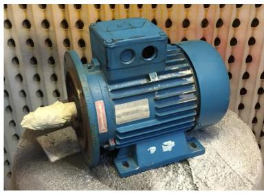
Figure 4.27 Motor prepared for primer and paint.
