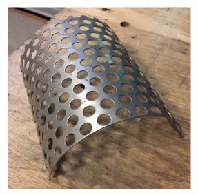
Figure 5.4 Sieve with a larger perforation.
