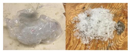
Figure 5.3 LDPE-film before and after being shredded without a sieve.
