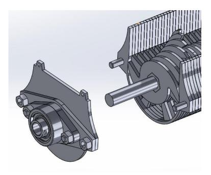
Figure 6.13 Final redesign - exploded view.
