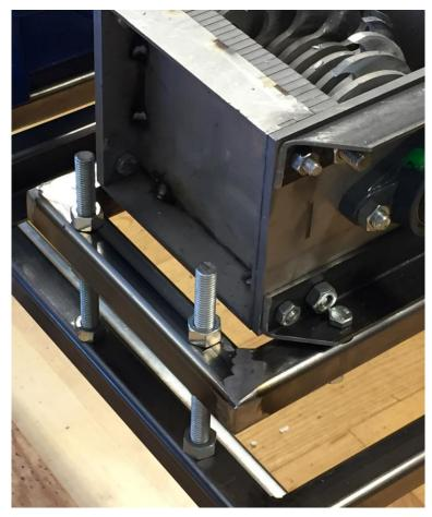
Figure 4.34 Adjustable framework solution for the SSP.
