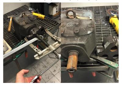
Figure 4.20 Successfully removing the pulley with an angle grinder.
