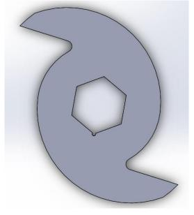
Figure 6.2 Redesigned knives with a straight leading face
