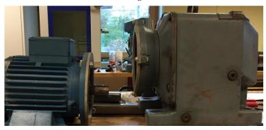
Figure 4.23 PSU configuration after removing the rotor with the remaining shaft connected to the gearbox.
