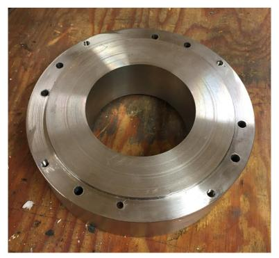
Figure 4.26 Lathed connection between motor and gearbox.
