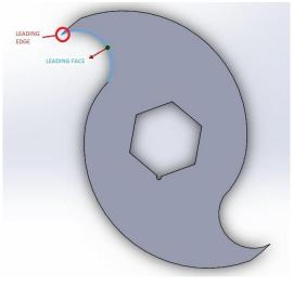
Figure 6.1 CAD view of Hakkes knives.
