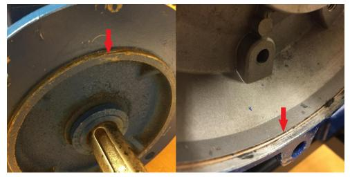
Figure 4.25 Spigot (left) and socket (right) of the flanges marked by arrows.
