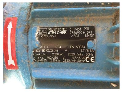
Figure 4.5 Rating plate of the motor.
