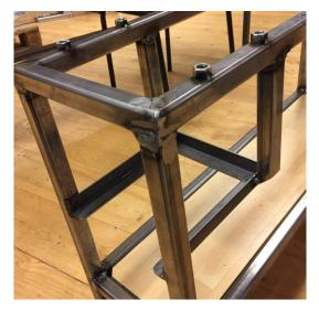
Figure 6.17 Slide rail for a smaller collector.
