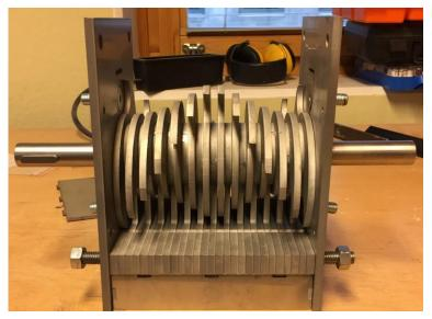
Figure 4.31 Knife configuration shaped like a V.
