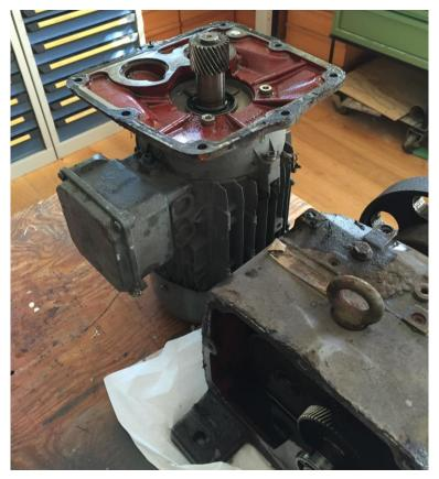
Figure 4.16 Motor separated from gearbox.
