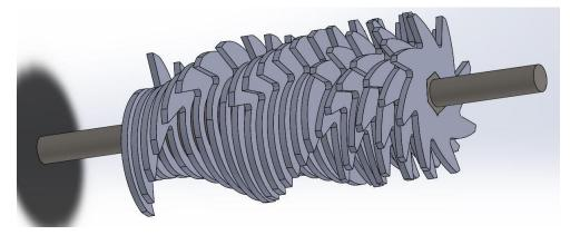
Figure 6.3 Extended shaft with increasing amount of teeth.
