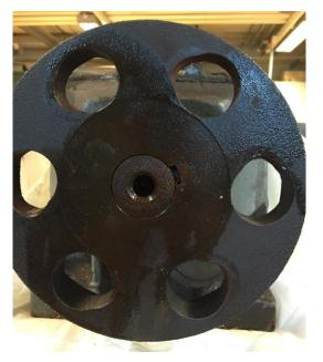
Figure 4.17 Pulley on the output shaft of the gearmotor.
