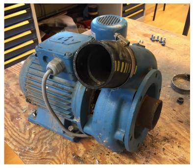
Figure 4.4 Used motor from a local junkyard.
