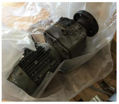
Figure 4.13 Gearmotor as found on the junkyard.
