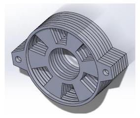
Figure 6.6 Integrated housing with spacers and counterknives.
