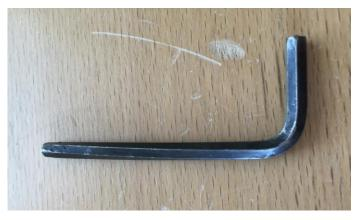
Figure 4.18 Allen key twisted from trying to remove the set screw.
