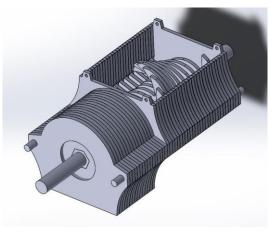
Figure 6.7 Extended infeed and modified housing.
