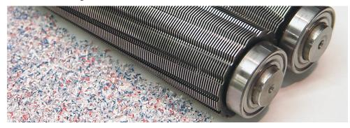
Figure 3.7 Paper shredder with hook knives.
