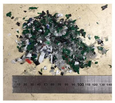
Figure 5.5 Output quality from a mixture of PP, PET and PS when using the sieve with larger perforation.
