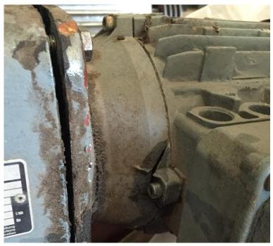
Figure 4.15 Damaged flange connection.
