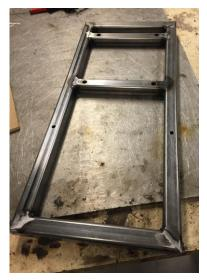
Figure 4.33 Detachable frame for the PSU.
