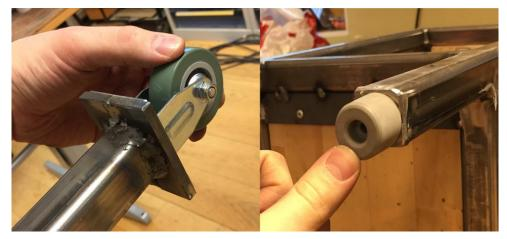
Figure 6.16 Redesigned feet of the framework.
