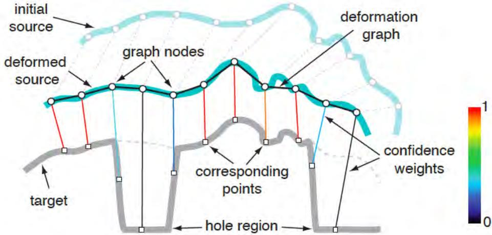
Figure 3: An illustration of the relation between the initial source scan, the deformed source and the target scan. The color of the confidence weights describe the correspondence between the deformation graph node and the target node [21].
