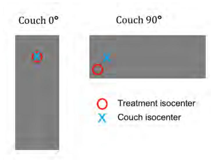
Figure 18: Illustration of the effect of a couch rotation offset.
