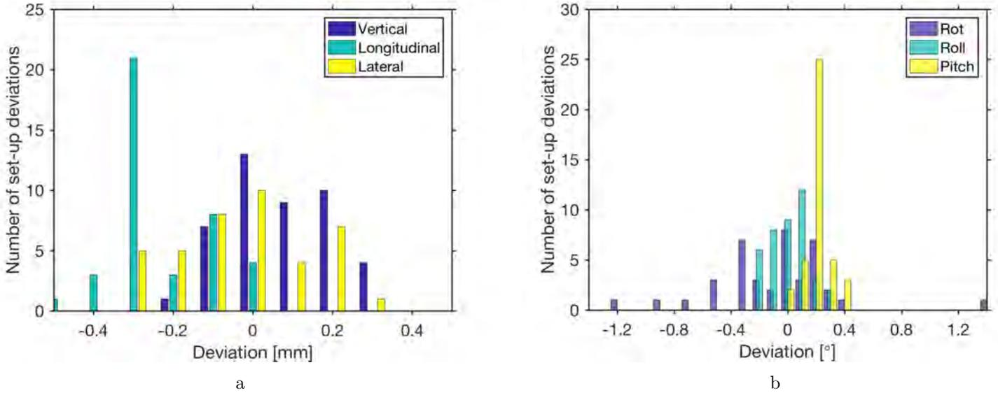
Figure 13: Total translational (a) and rotational (b) set-up deviations for all four PTVs (with different isocent positions), with an OSS-based set-up at couch angle  $0^\circ$ .
