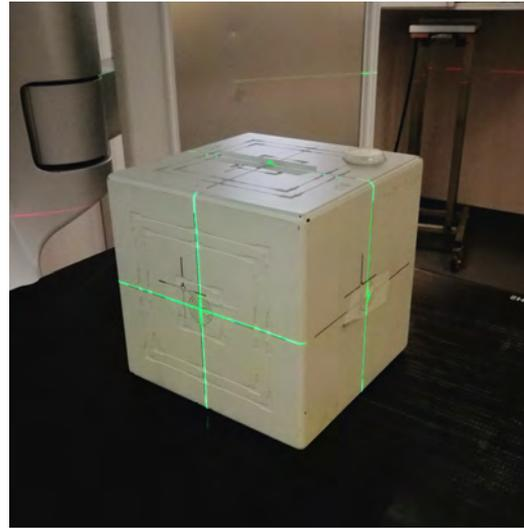
Figure 4: The QUASAR™ Penta-Guide Phantom used for the Routine QA.
