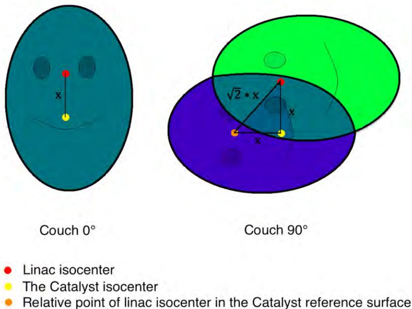
Figure 17: Illustration of the effect of a misalignment between the treatment isocenter and the OSS systems isocenter when rotating the couch [22].
