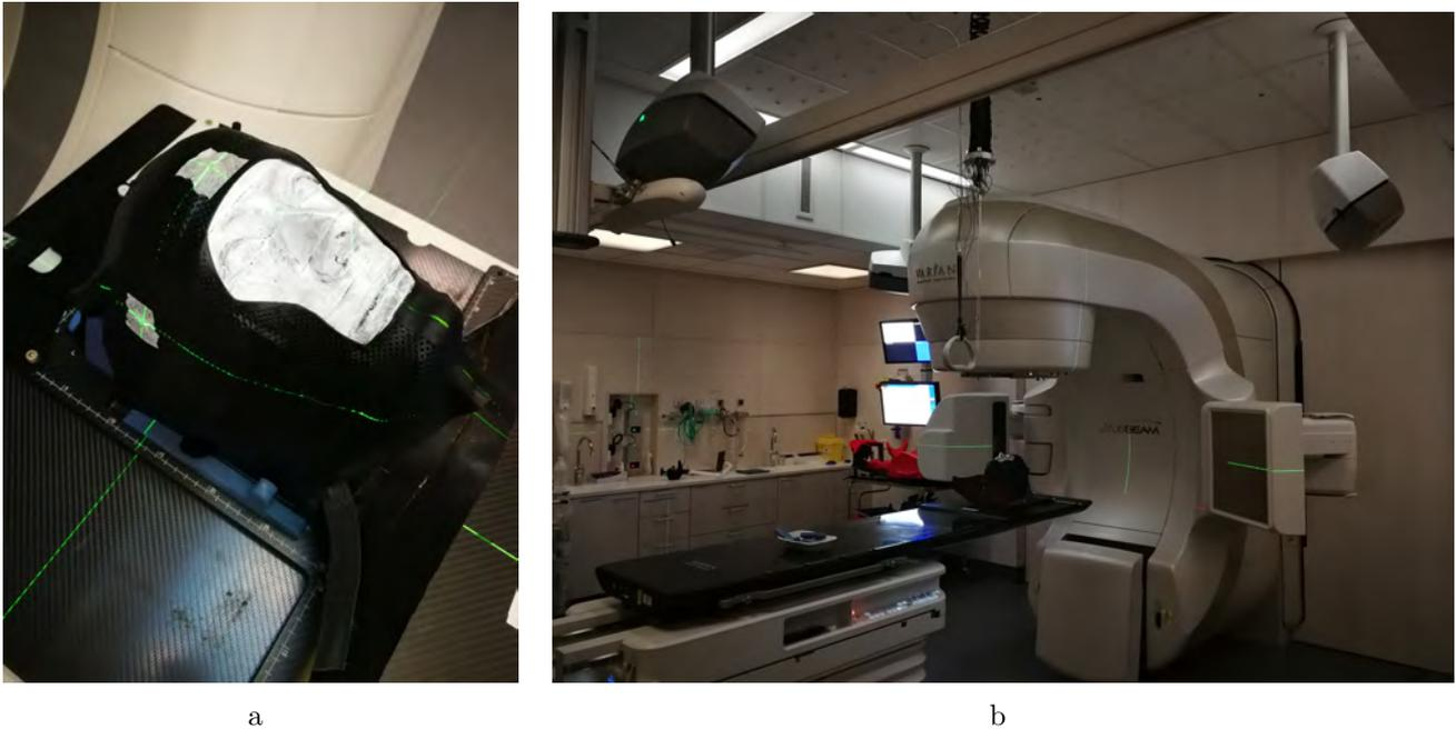
Figure 8: The Alderson RANDO Phantom immobilized with an open-face mask (a) and the treatment room with a Varian Truebeam linear accelerator and the ceiling-mounted three-camera OSS system (b).
