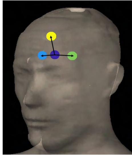
Figure 9: Four PTVs placed in different parts of the brain of the Alderson RANDO phantom.
