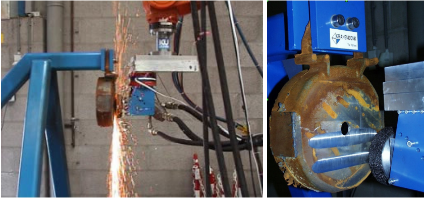
Figure 3.3 Grinding with Irb 6400 industrial robot, constant force reference of 150 N.
