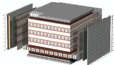
Fig. 1. Each calorimeter tower consists of 8 layers of 12 CsI(Tl) crystals stacked in an x - y configuration. A calorimeter tower contains 96 crystal logs and measures about 40 \times 40 \times 20 \text{ cm}^3 . In total there are 1536 crystals.
