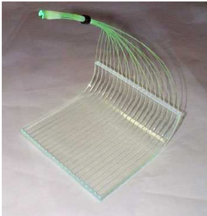
Figure 3.3: A photo of one of the plastic scintillator tiles used in GLAST together with the wave-shifting fibers to be connected to the PMT used for readout. Photo taken from [19].
