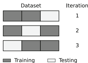
Figure i.8: Illustration of a K-fold cross validation with K = 3 . The dark gray boxes correspond to the training data and the light gray to the data that will be used for testing.
