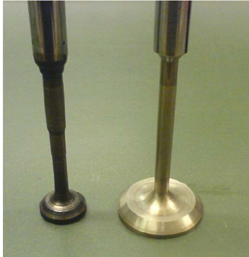
Figure 44 Picture illustrating the difference between the “small tank valve” ( \varnothing = 16 mm) and the “large tank valve” ( \varnothing = 28 mm).
