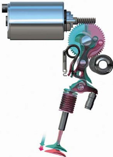
Figure 17 Illustration of BMW's Valvetronic mechanism [33].
