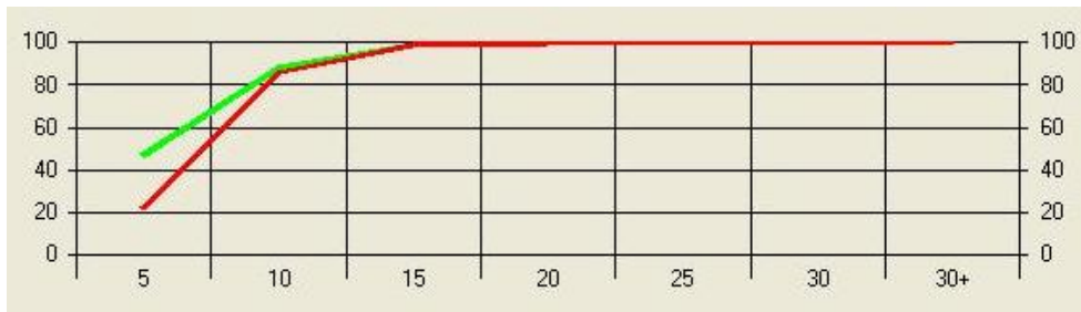
Figure 5 The level of coverage (in percent) for the risk category of single car accident shown as a function of response time (minutes). The top graph shows the situation for the current organisation (daytime) with only stationary units. The bottom graph shows the level of coverage for a scenario using mixed stationary and non-stationary units. The red line shows the normal case and the green line the most favourable case.
