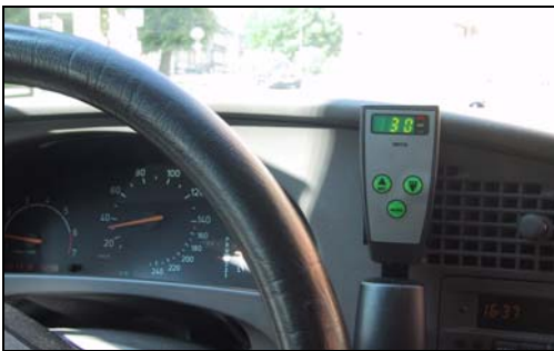
Figure 2: The display showing the current speed limit. (Published with the kind permission of SG Utveckling)
