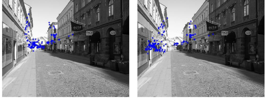
Figure 5: The reprojection of visible 3D points when the (1,3) solver (left) and the six point solver (right) is used. In this example Model 1 is used and all points in front of the camera are reprojected. The (1,3) solver has a correct position but the six point solver has not.
