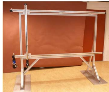
Fig.3. The experimental setup xy-table, with x and y travelling ranges of 2 and 1 meter, respectively.
