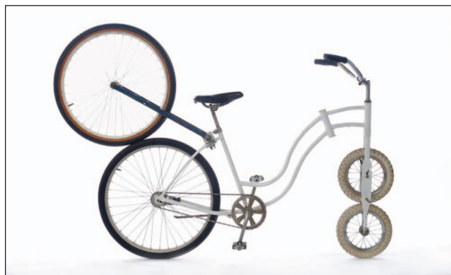
Figure 12. The UIUC naïve bicycle with precession canceling. This bicycle is used to demonstrate that a bicycle is rideable even when there are no gyroscopic effects. The bicycle is similar to the bicycle in Figure 11 but has a vertical front fork ( \lambda = 90^\circ ) and zero trail ( c = 0 , see Figure 1), which means that the front fork does not turn when the bicycle is tilted.
