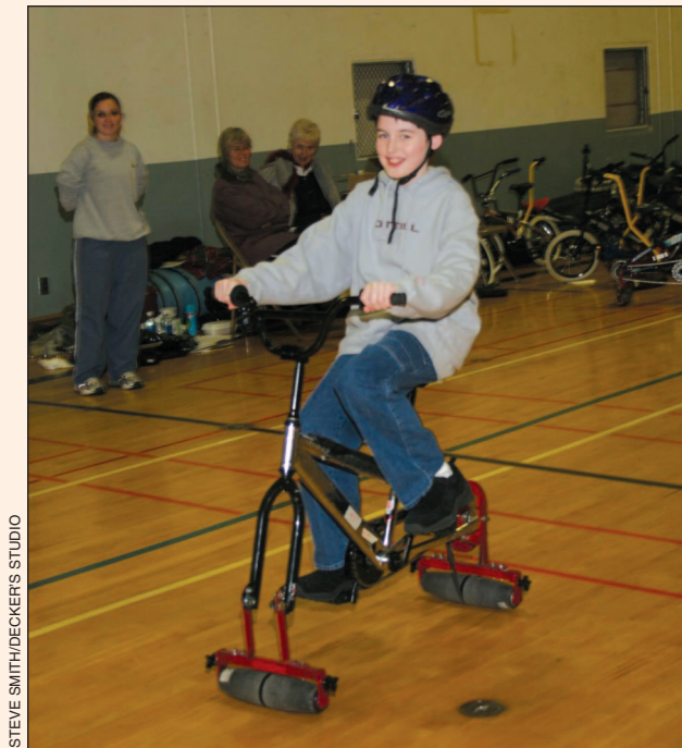
Figure 22. A child on an entry-level adapted bicycle. The wheels are replaced with crowned rollers. Virtually all children love the idea of being independent bicycle riders. This child rides comfortably because the bicycle is stable. As the child becomes more proficient, we substitute rollers with more crown (smaller R in Figure 21) and eventually transition the children to conventional bicycles.
