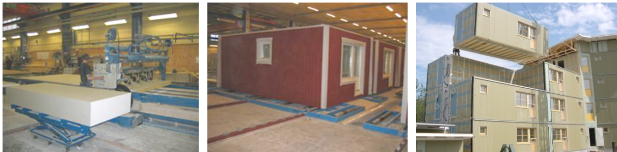
FIG 2: Modular house production
