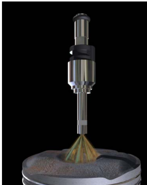
Figure 40: Fuel spray during the negative valve overlap
