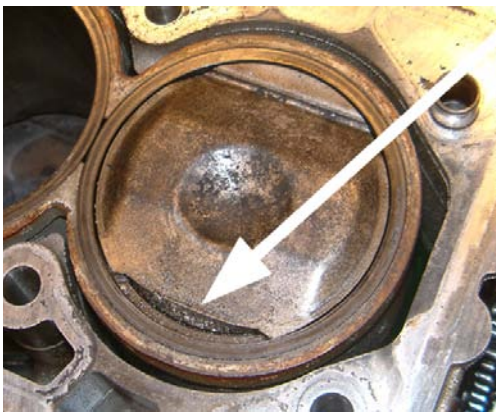
Figure 42: Damaged piston due to high PCP
