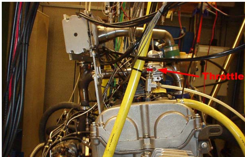
Figure 16: Throttle controlled intake temperature
