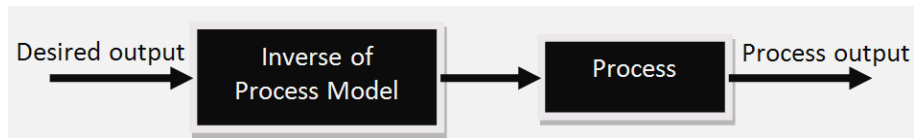
Figure 33 Ideal model-based control block diagram
