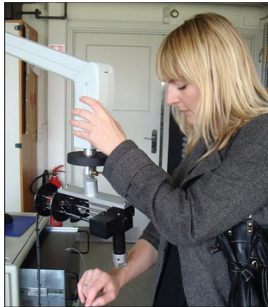
Figure 4.4: The probe was mounted on a supporting arm for stabilization and to reduce noise induced by unwanted probe-sample inter movement, here demonstrated by an OCT model.
