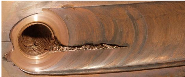
Figure 4-1. Visible wormhole during lid weld at TWI.
