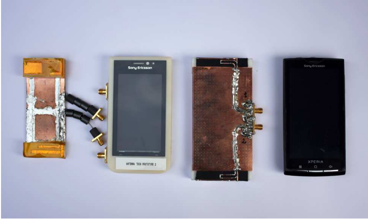
Figure 1.2: From the left: three representative multiple-antenna prototypes evaluated in this thesis. First from the right: a Sony Ericsson Xperia10 smart phone shown for size comparison.
