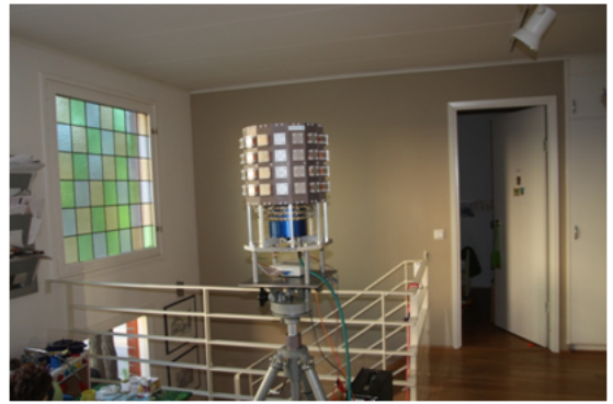
Fig. 3. 128-port receive antenna in the upstairs position.
