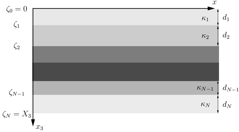
Figure 4.8: The acoustic scattering geometry for a layered medium.
