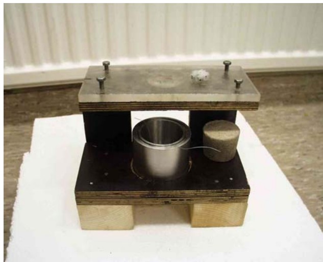
Figure 4.9 Some specimens of those \phi 45 mm in diameter were cast with steel fibres of only 0.7 mm in diameter sticking through them. After demoulding, the steel fibres were removed, leaving thin holes through the specimens. The wire in the figure is not stretched as it would be during casting.
