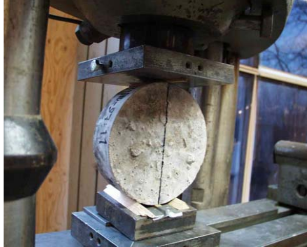
Figure 4.21 Splitting test of a concrete specimen.
