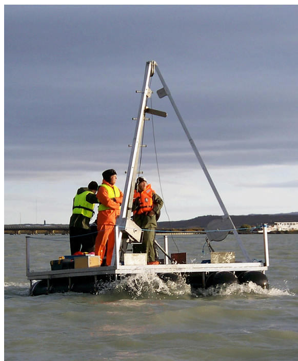
Figure 2. Uwitec floating platform used during core collection in Lake Lögurinn.
