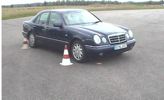
Figure 2.4 The \mathcal{H}^2\mathcal{C} test vehicle. It is a modified Mercedes E220 passenger vehicle, fitted with an advanced brake-by-wire system and four state of the art electro-mechanical disc brakes.
