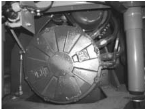
Figure 10: An water-cooled induction machine.
